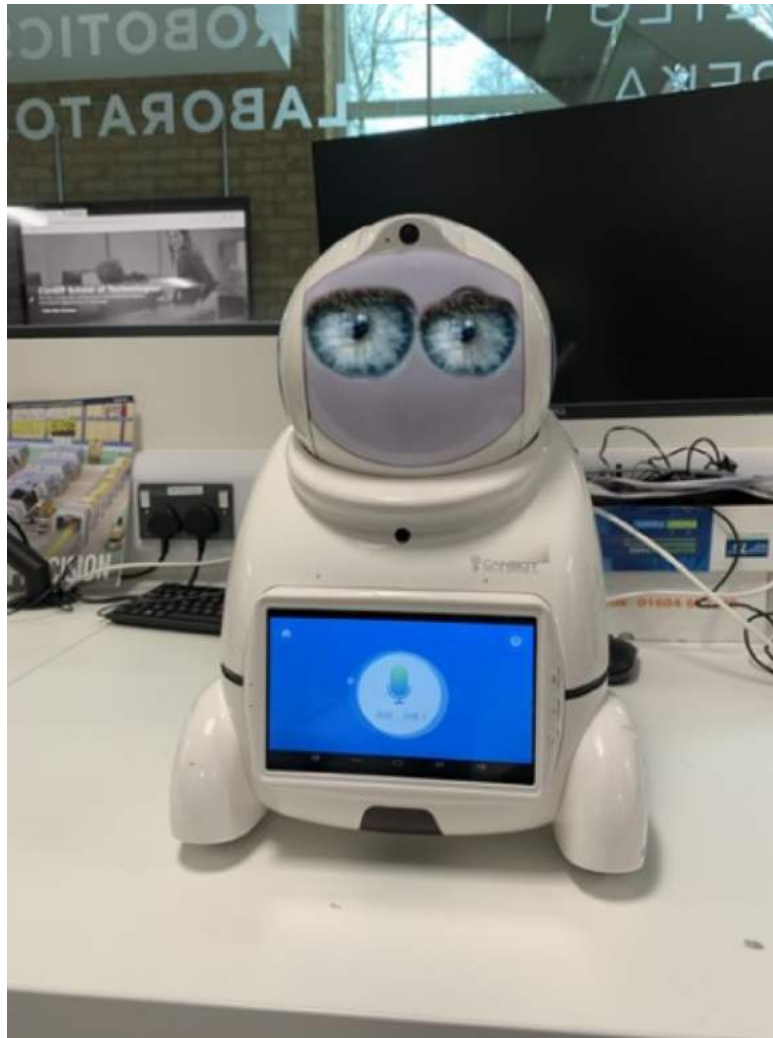
Figure 2 Canbot-U03 robot with human eyes modification.
